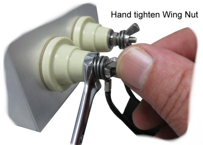
Using 3/8" wrench - hold hex nut steady
