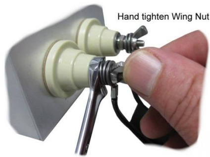
Using 3/8" wrench - hold hex nut steady
