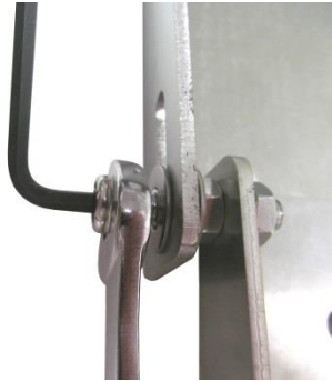
Using the Allen wrench and 1/2" hex wrench
