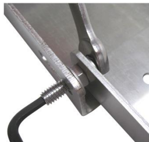
Allen Wrench and 1/2" open end wrench
