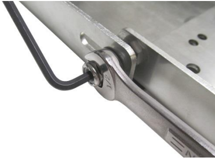
Using the Allen wrench and 1/2" hex wrench
